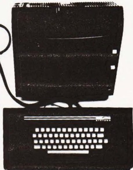
NBZ80-HL. As NBZ80-S, with 16k bytes of RAM, expansion board with 8k BASIC ROM, video interface board, alphanumeric keyboard, book "BASIC Programming Primer". (TV monitor is optional).
